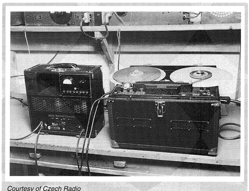
Figure 6 A portable tape recorder of the 1950s, the AEG Magnetophon K4.
